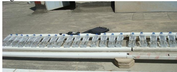
Figure 2) SODIS and KPS associated SODIS reactors configuration
