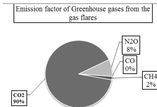
**Figure 3.** Comparison of greenhouse gas emission factors due to the activity of gas flares in Ahvaz oil field
