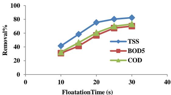
Figure 5) Effect of flotation time different on DAF in removal COD, BOD<sub>5</sub> and TSS
