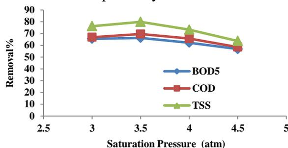
Figure 6) Effect of saturation pressure different on DAF in removal COD, BOD<sub>5</sub> and TSS
