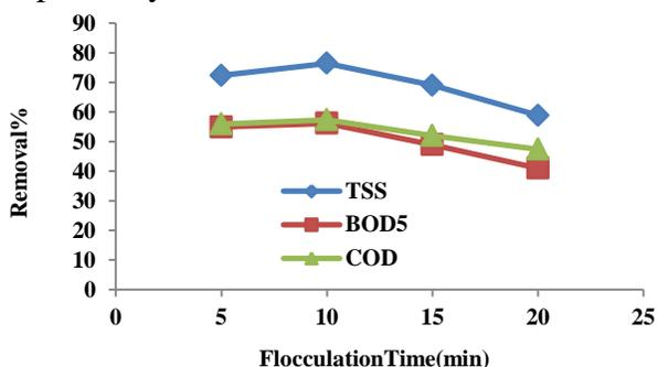
Figure 4) Effect of flocculation time different on DAF in removal COD, BOD<sub>5</sub> and TSS
