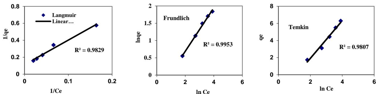
Figure 6) Isotherms adsorption of pCNB onto MSW
