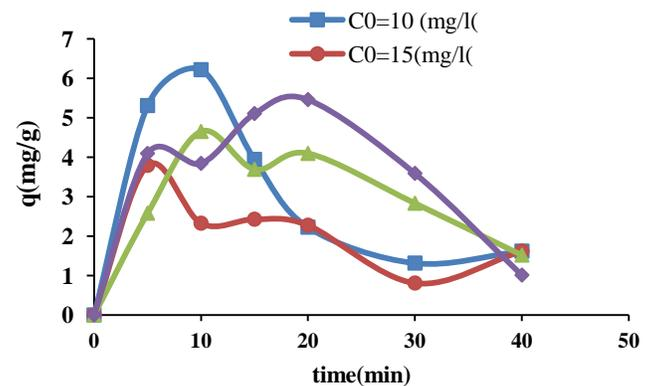
Figure.2) Effect of initial concentration and contact times on NOMs adsorption capacity of walnut shell modified by ZnO with time
