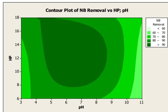
Figure 4) Contour plots of nitrobenzene removal in terms of pH and hydrogen peroxide concentration ( $C_F = 1.40 \text{ mM}$ ,  $T = 25^{\circ}\text{C}$ , and  $t = 30 \text{ min}$ )
