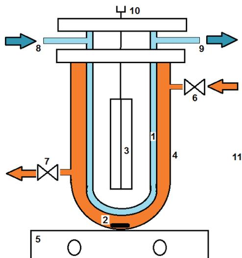
**Figure 1) Experimental setup in laboratory scale: 1) cooling water jacket, 2) magnetic stirrer bar, 3) UV lamp, 4) glass reactor, 5) magnetic stirrers, 6) input wastewater, 7) output wastewater, 8) cooling water input, 9) cooling water output, and 10) electric connection**
