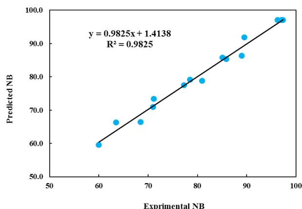
Figure 2) The predicted versus experimental values in the removal of nitrobenzene
