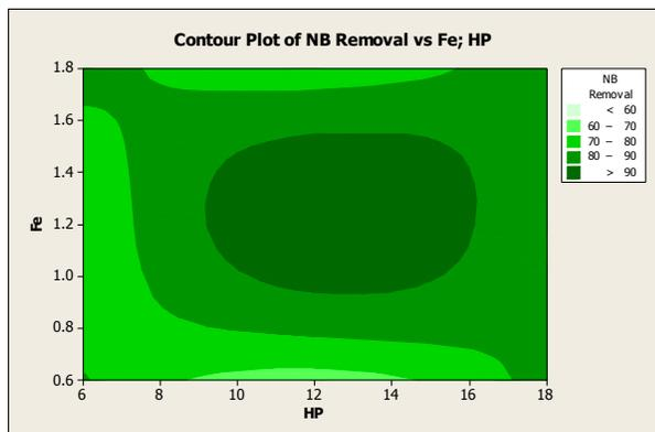
Figure 3) Contour plots of nitrobenzene removal in terms of Ferric ion and hydrogen peroxide concentration ( $T = 25^{\circ}\text{C}$ ,  $\text{pH} = 4.0$ , and  $t = 30 \text{ min}$ )
