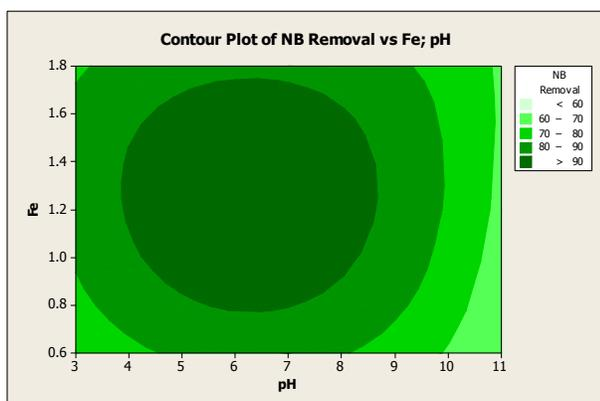
Figure 5) Contour plots of nitrobenzene removal in terms of Ferric concentration and acidity ( $C_{\text{HP}} = 20$  mM,  $T = 25^\circ \text{C}$ , and  $t = 30$  min)
