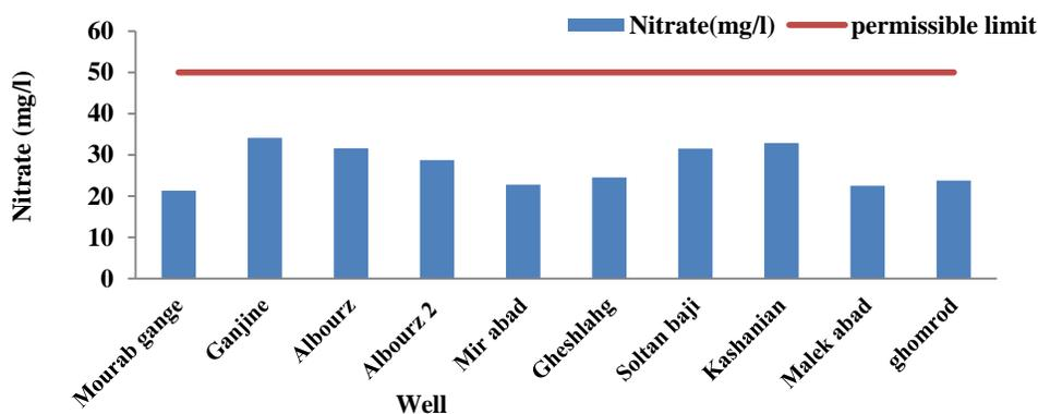
Figure 1) Concentrations of NO<sub>3</sub><sup>-</sup> in groundwater samples and comparison with permissible limit of Iran national drinking water standard
