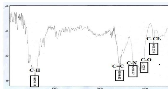
Figure 2) FTIR Spectrum of modified almond shell charcoal with ZnCl<sub>2</sub>
