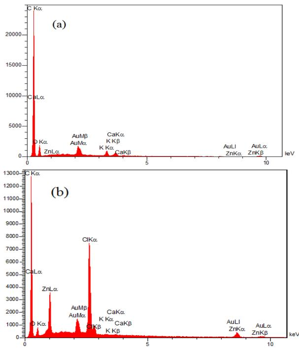
Figure 3) EDX analysis of charcoal almond shell a) before activation b) after modification with zinc chloride
