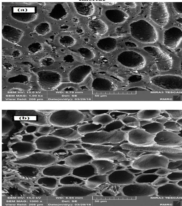
Figure 4) FESEM image of a) raw charcoal, b) modified charcoal with zinc chloride
