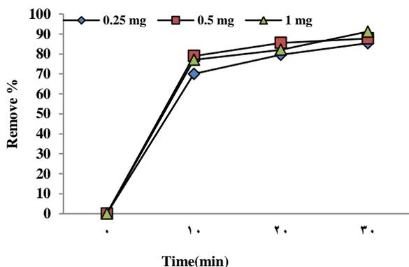
Figure 2) The effect of contact time on dye removal efficiency by granular pumice (pH=3)
