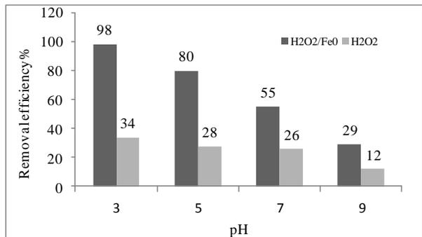
**Figure 4: Effect of pH on the efficiency of the process (dye concentration = 50 mg/l, contact time = 80 min, Fe nanoparticles concentration = 2g, hydrogen peroxide concentration = 200 mmol/l).**
