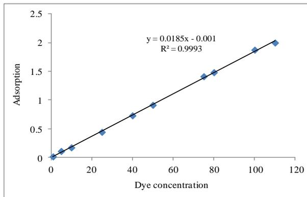
**Figure 3: Calibration curve for measuring Acid Red 18 concentration**
