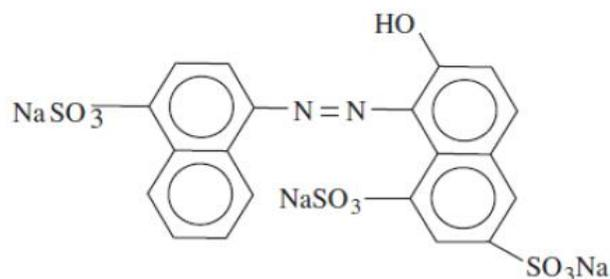
Figure 2: chemical structure of Acid Red 18
